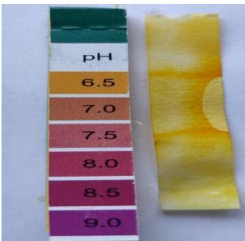
Figure 9. Test for pH for lotion.
